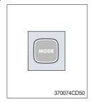
Operating this switch, it beeps and displays symbol of each mode in order. (Vent/Foot → Def/Foot → Def/Vent → Def/Vent/Foot)
